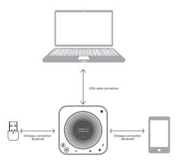
Support USB, dual Bluetooth multi-channel data fusion, can realize three connection methods to work at the same time, so that it can support simultaneous access to multiple parties for conferences;
