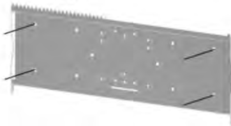
Mounting back plate to the wall
