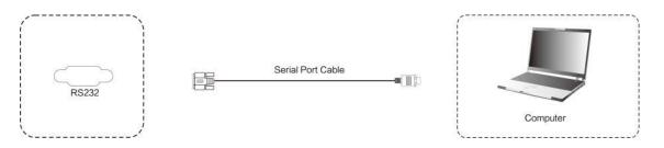
After using serial port cable to connect central control equipment and machine, certain function of the machine can be controlled via central control equipment, such as: machine ON/OFF, and adjustment of sound volume, etc.
