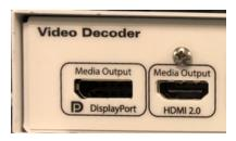
The ZyPer4K Decoder device can be ordered with an optional DisplayPort output.
