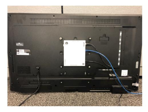
Example mounting ZyPerK to side of 200x200 VESA bracket using 2 mounting holes/screws. This *may* enable use of wall mounting bracket hardware.
