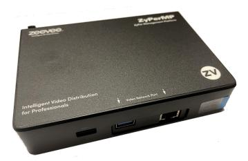
Most installations will require a ZyPer Management Platform (ZyPerMP). This device controls the operation and manages the connectivity between endpoints. The management platform is a hardened controller node that must reside on the same logical network as the ZyPer4K Encoders and Decoders. It runs a ZeeVee application as its sole function. The application presents an API to potential third party management platforms as well as hosting its own management application.
