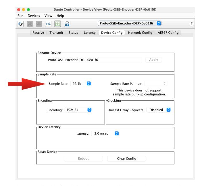
Incorrect setting of the **Sample Rate** field will cause a Dante Transmitter to not see audio as available to transmit.
