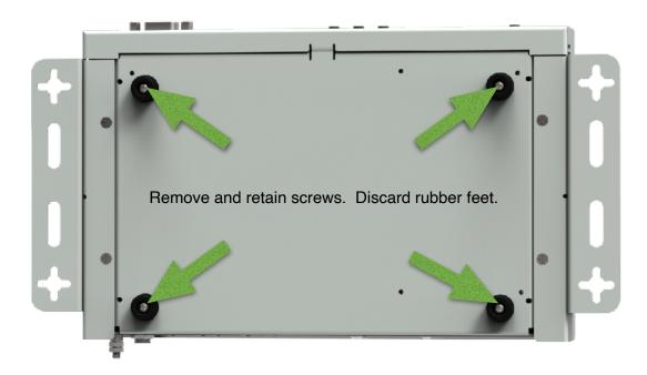
Affix the L-Brackets to the sides of the unit using the retained screws from the rubber feet (repeat for each side).
