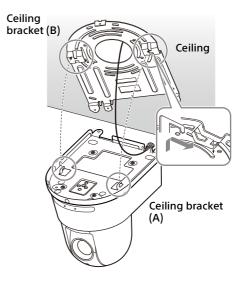
5 While pushing up the entire camera, attach it to the ceiling bracket (B) using the 3 supplied screws (M3 × 8).
