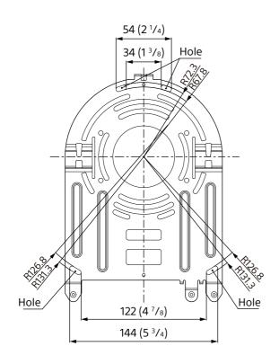
With the ceiling bracket installed
