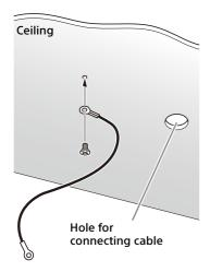
1-2 In the case that a wire cannot be attached on the ceiling, attach the wire on the ceiling bracket (B) as illustrated below with the supplied screws (M3×8).
