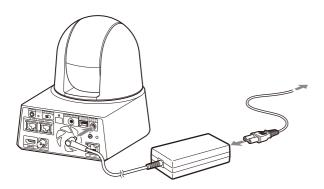
2 Fix the AC adapter cord with the cord clamper so that it does not come out. Unlock the cord clamper and put the cord through it.
