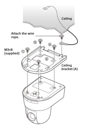
Lightly tighten screws temporarily in the order indicated in the figure. Afterwards, screw each of them firmly.
