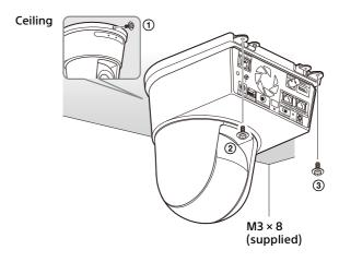
Lightly tighten the screws temporarily in the order indicated in the figure. Afterwards, screw each of them firmly.
